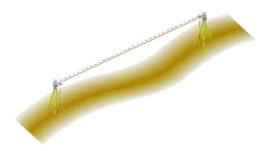
Reciprocal Vertical Calculations improves elevation accuracy by averaging two opposing measurements.
