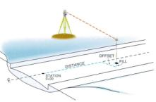
out, the SDR33 will give you angles and distances to set out that point in 3-D. Horizontal and vertical offsets and checking of roads under construction may also be easily accomplished with this program.
