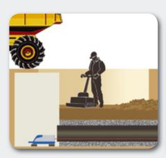
LINE ALERT: This unique feature is ideal for working in high-vibration or wet conditions where the pipe lasers may be disturbed. The beam flashes to notify you that the setup line has been disturbed, eliminating the necessity of rework. Combined with the self-leveling warning, you'll always complete the job correctly, on time and on budget! Only available on the DG711.
