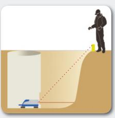
LINE SET: The Line Set/Check capability of the pipe laser allows you to raise the beam outside of the trench for fast line setup or checking. Raising the laser beam out of the trench to an above-ground stake saves you time—instead of having to move the excavator off line during setup of the pipe laser, you can just get on with your job. In addition, the Line Set-Check feature is ideal for rechecking the line in pipe jacking puts after each push. Only available on the DG711.
